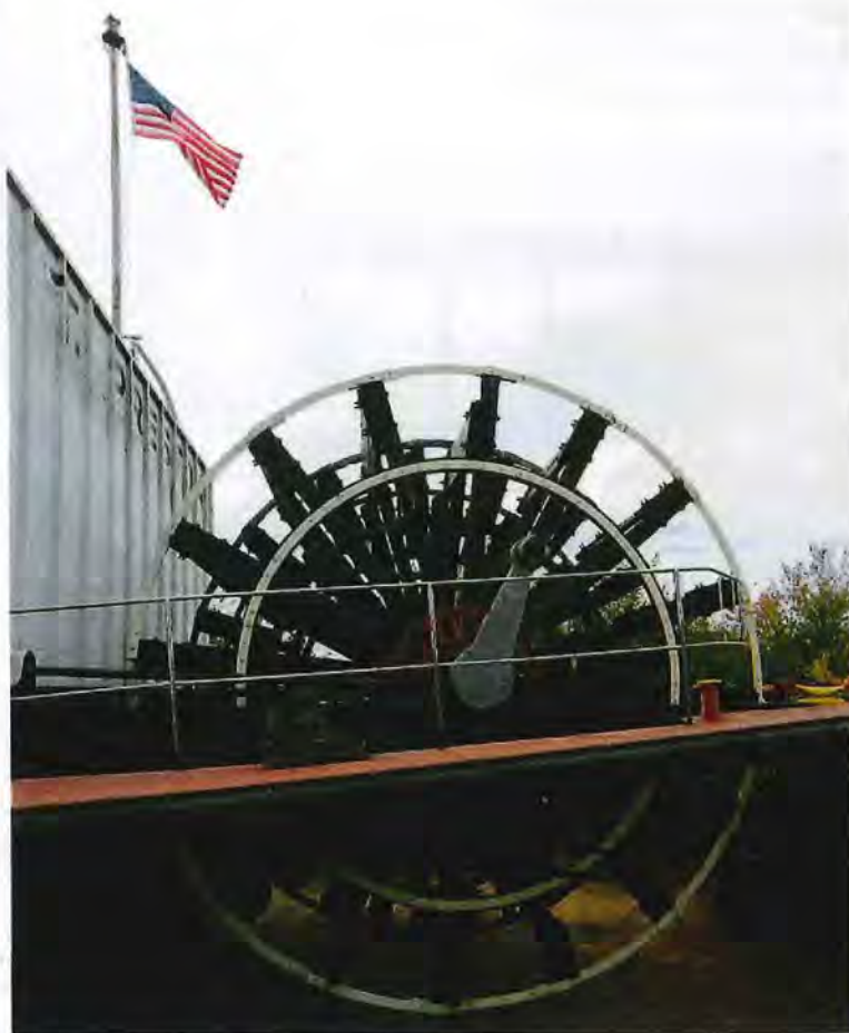
Old-school power: The wood-planked paddle wheel of the W.T. Preston snagboat on Sixth Street in Anacortes is 17 feet in diameter. The Preston, the last stern-wheeler to work Puget Sound, retired from duty in 1981.
