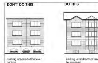
Example design standards for in-structure parking.
