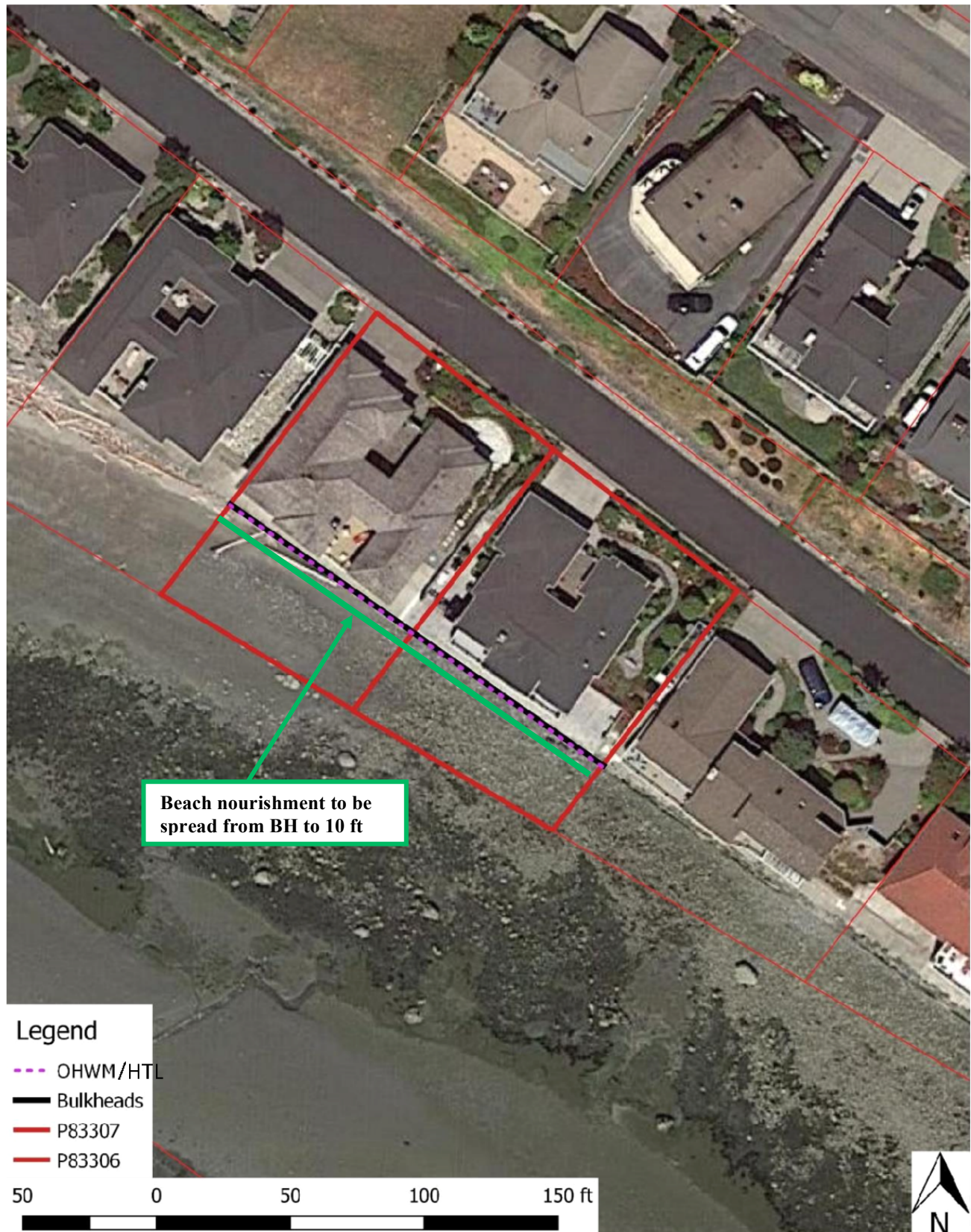
Figure 1. Overall site plan showing beach nourishment placement
