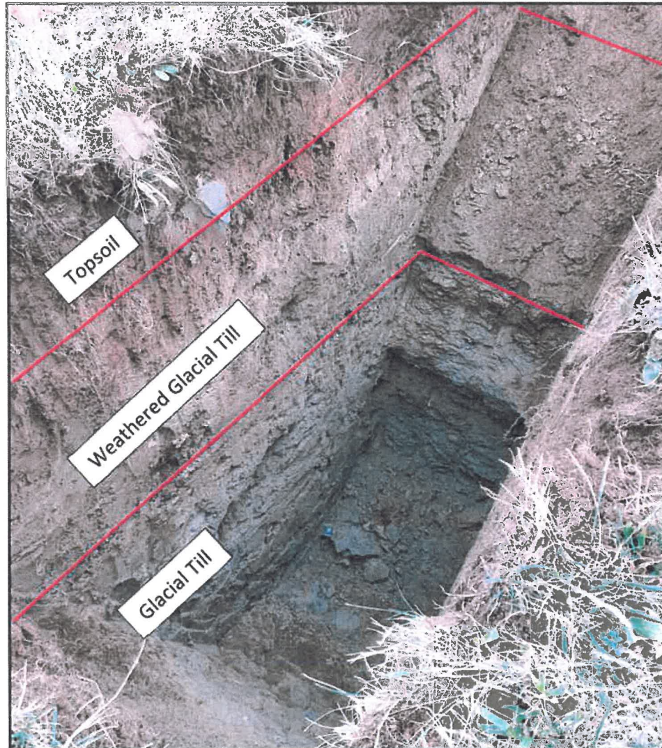
Image 2. View of test pit 3 (TP-3) showing the typical subgrade soil profile for the project site.
