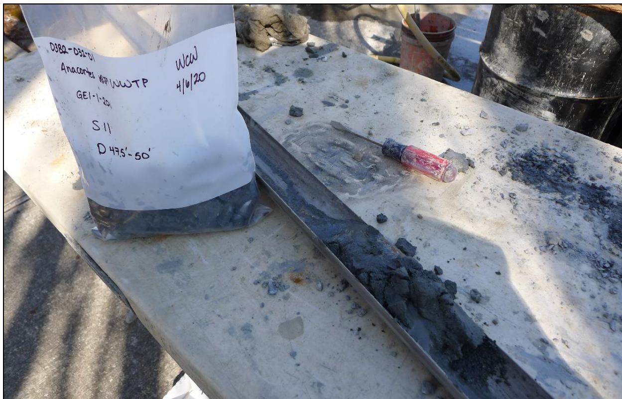
Photo 2. An example of the collection process from auger to bag.
