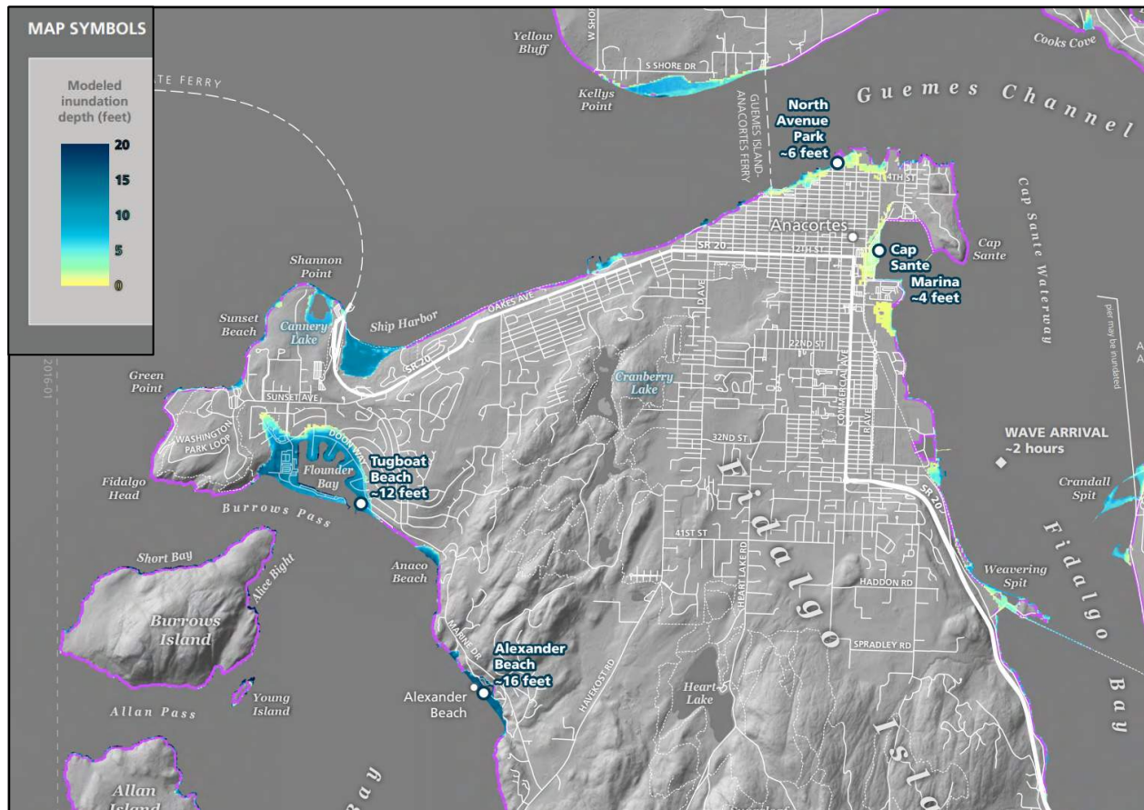
Figure 13. Tsunami inundation map of Anacortes with estimated arrival time and predicted inundation depth points. Data from Eungard et al. (2018) for the CSZ L1 magnitude 9.0 earthquake scenario. Purple line indicates where shoreline inundation is inferred but not quantified.
