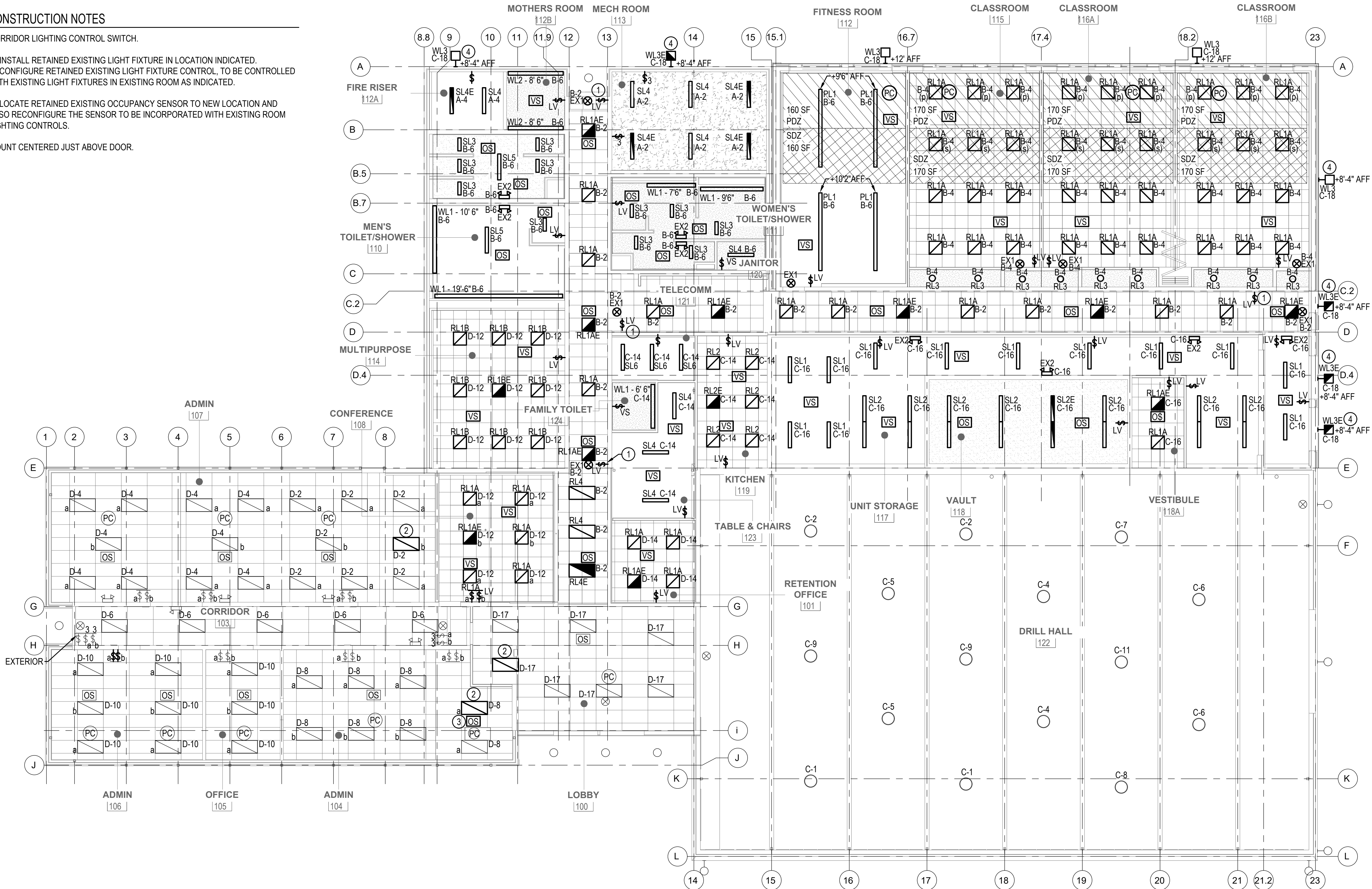
① ELECTRICAL LIGHTING PLAN SCALE: 1/8"=1'-0"
