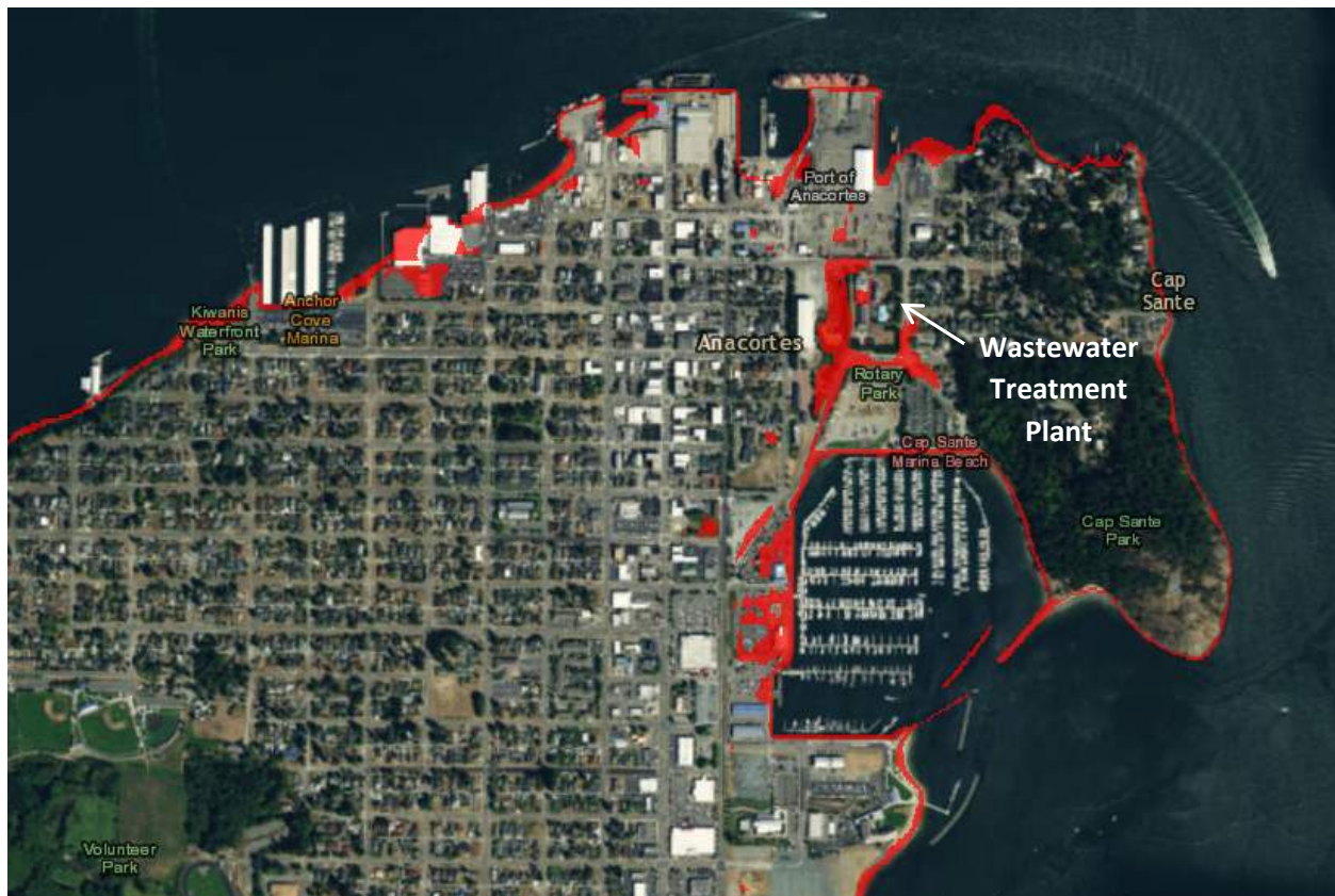
Figure 3. Low-lying areas currently subject to shallow coastal flooding. The wastewater treatment plant is in a particularly vulnerable area. Note: data are based on local tidal height thresholds from a three year average between 2007 and 2009; current conditions may be different for specific areas (NOAA, 2016).
