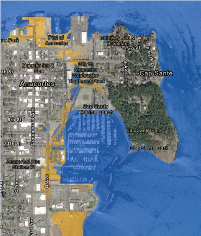
Figure 5. Inundation extent for SLR above base flood elevation (BFE) for downtown Anacortes.
