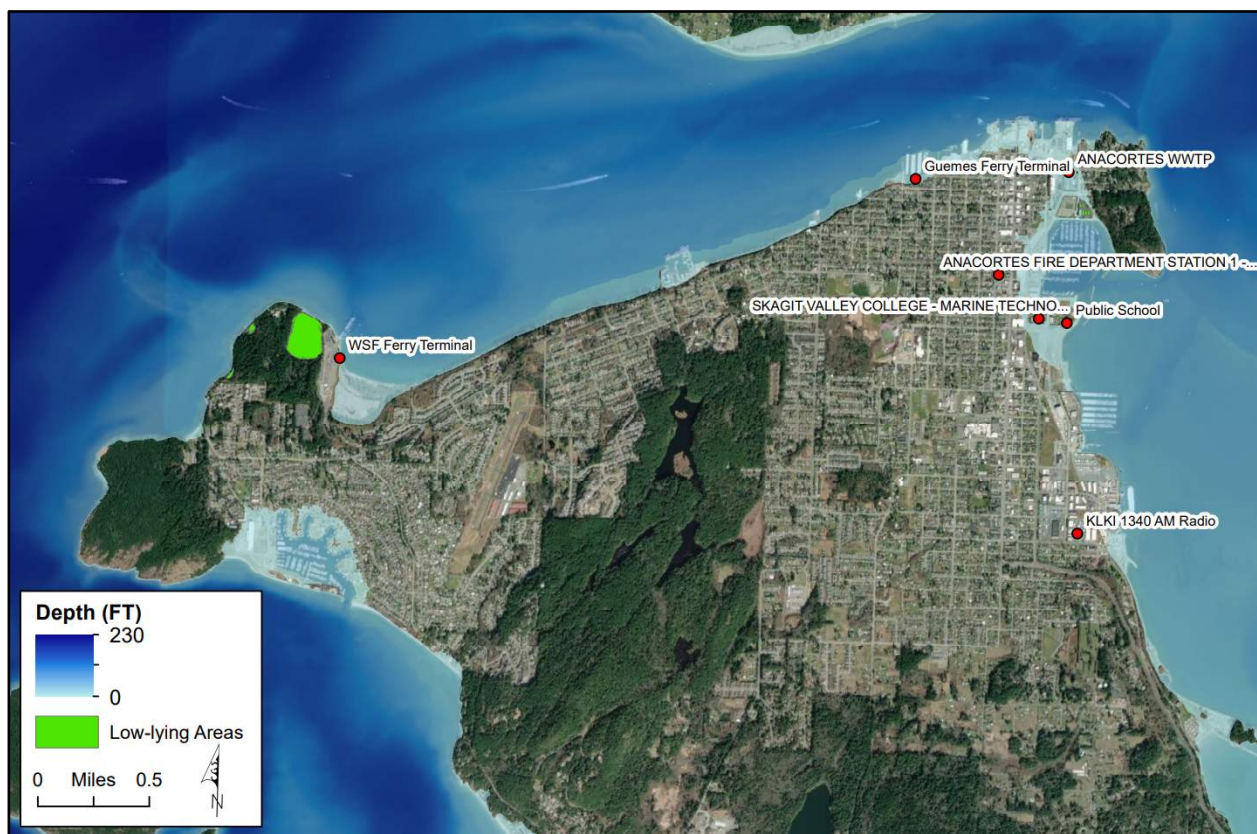
Figure 15. Critical infrastructure within or near the 2100 high emissions sea level rise scenario. Light blue areas would be inundated in this scenario, and the “low-lying area” is not mapped as connected to saltwater (due to the old railroad causeway at Ship Harbor). Data from HAZUS and WA Geospatial Open Data portal.
