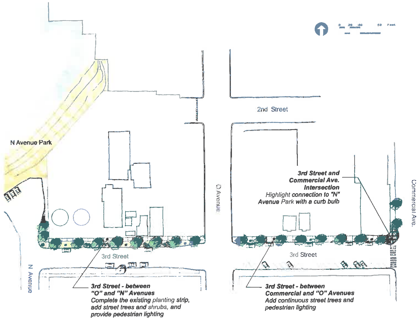
Figure 51. Connection to "N" Avenue Beach Improvements Plan
