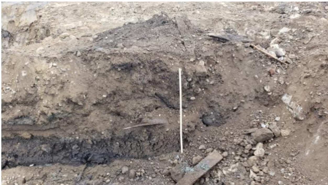
Figure 22. Historic debris throughout fill layer (Note “peat” layer at base of cut).
