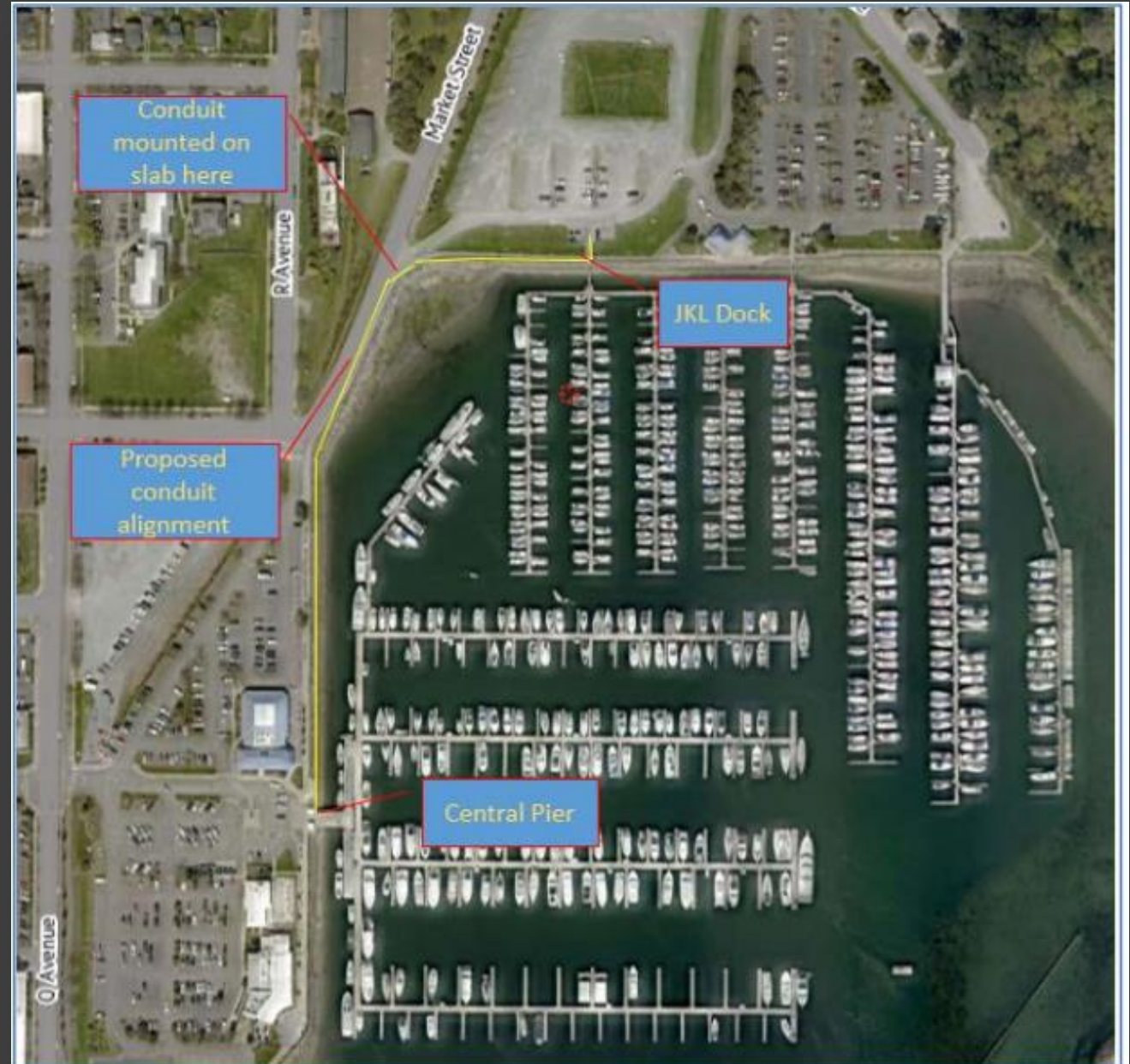
Figure 1: Fiber conduit route at Cap Sante Marina
