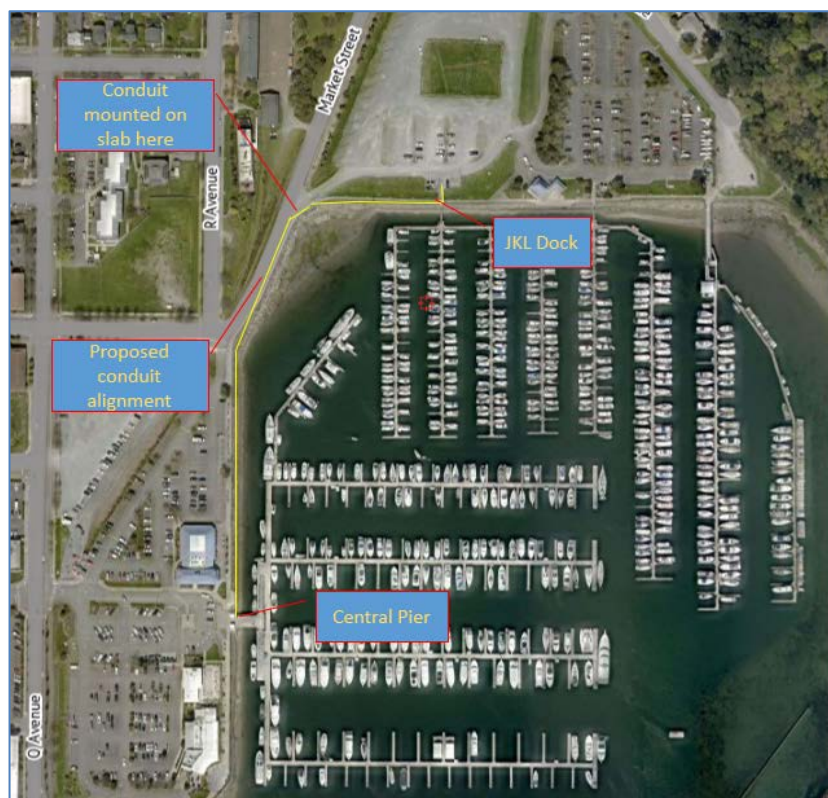
Figure 1: Fiber conduit route at Cap Sante Marina
