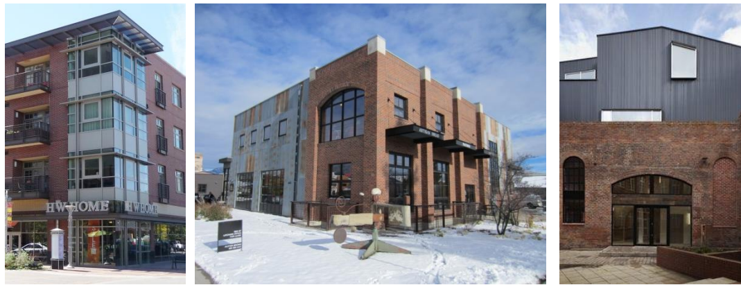
Figure 19.63.050(C)(2) Acceptable metal siding examples
