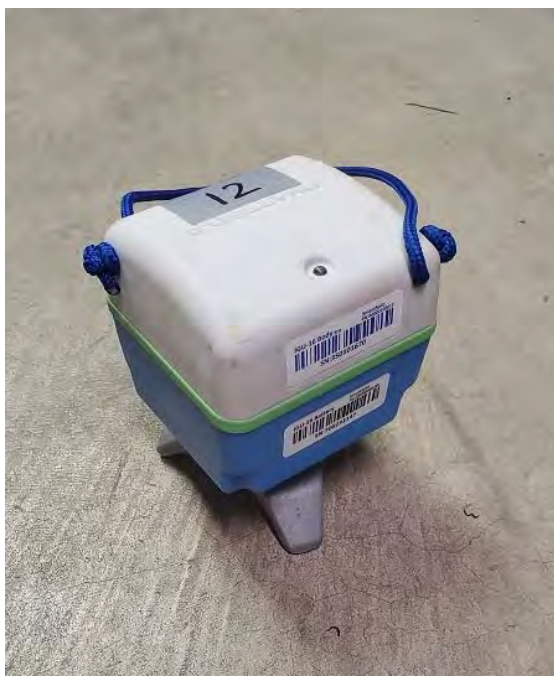
Figure 2. SmartSolo IGU-16 wireless sensor
