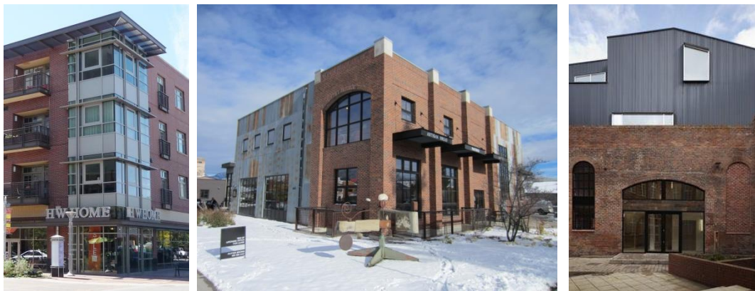
Figure 19.63.060(C)(2) Acceptable metal siding examples
