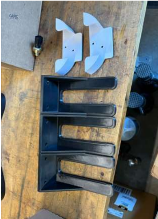
Custom tool holders, printed in-house
