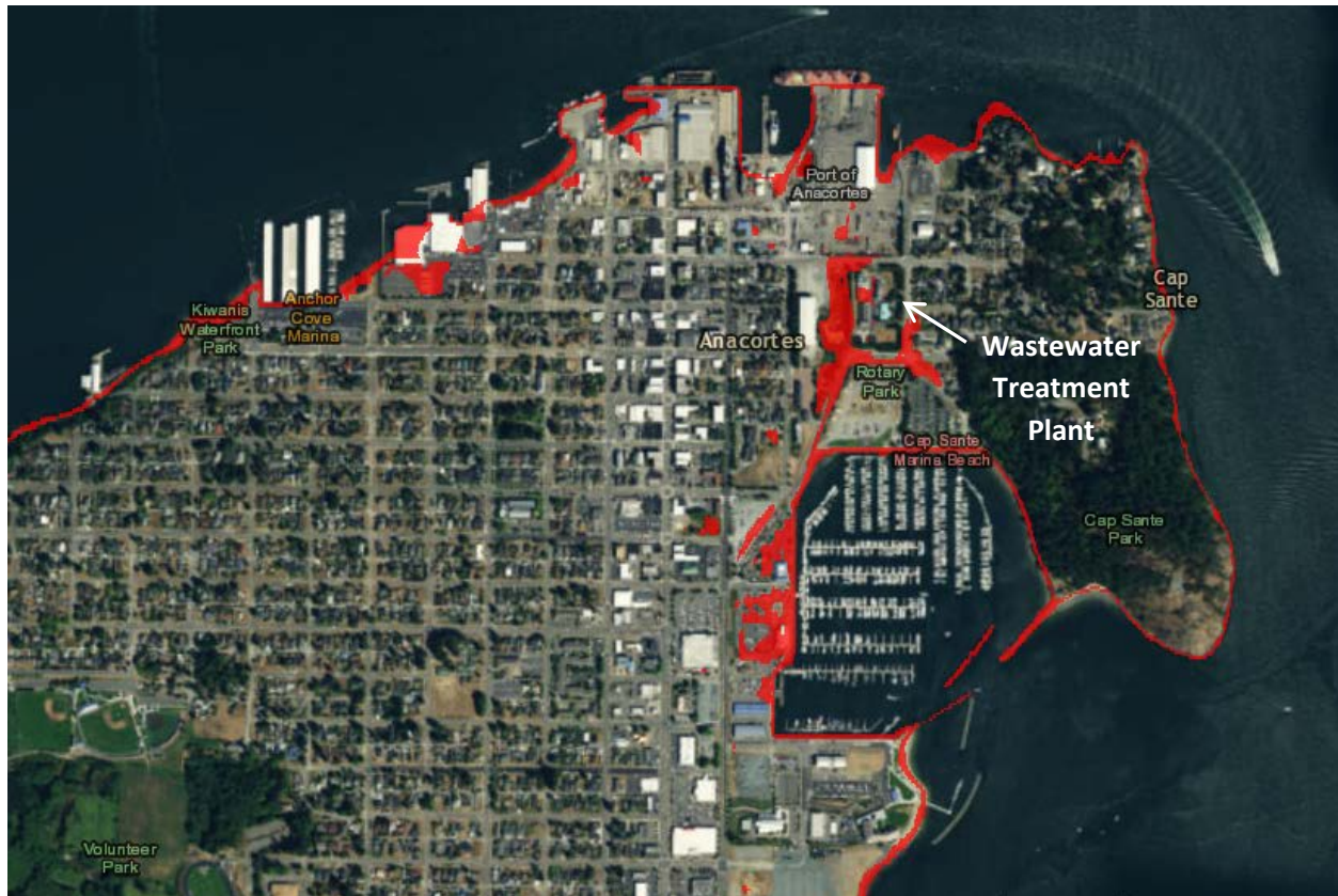
Figure 2. Low-lying areas currently subject to shallow coastal flooding. The wastewater treatment plant is in a particularly vulnerable area. Note: data are based on local tidal height thresholds from a three year average between 2007 and 2009; current conditions may be different for specific areas (NOAA 2016).
