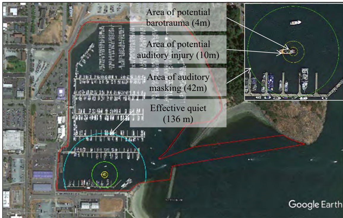
Figure 4. Approximate area of potential marbled murrelet injury/auditory masking threshold exceedance (yellow) from pile driving.
