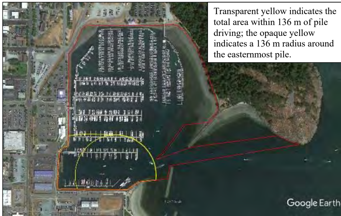
Figure 3. Approximate area of potential salmonid cumulative noise threshold exceedance (yellow) from pile driving
