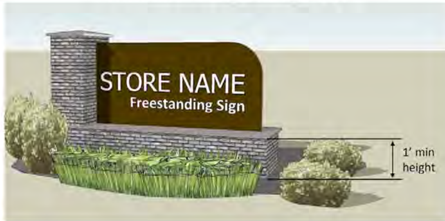
Figure 19.67.070(C)(4) Minimum base height for sign copy.
