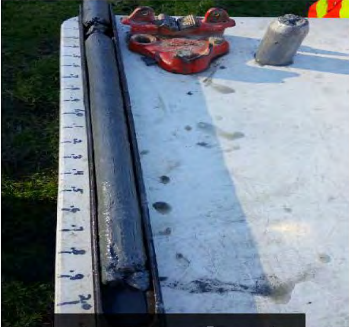
Photo 2: Core from geotechnical boring location shown in Picture 1 above, showing native soil and no indication of contamination was noted.
