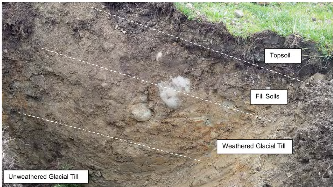
Photo D: South side of excavation at TP-2. Soil units and approximate contacts labeled.
