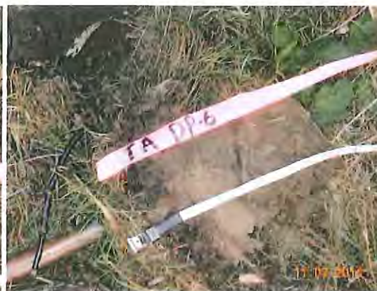
Photo 4 – View of soil profile at upland data point 6 showing lighter brown matrix and absence of redoximorphic features.
