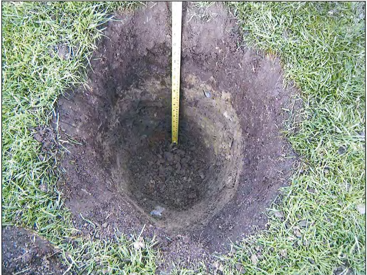
Photo 5. Typical soil profile observed at the project site (OP-1).
